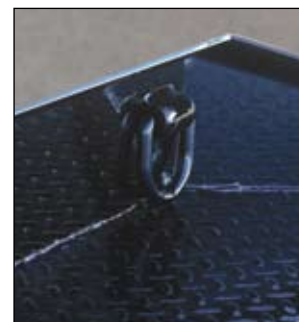
5K Lbs. D-Ring tie Downs – At each corner provide easy load securement.
