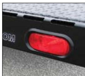
Sealed Lights – DOT approved lights and reflective tape.
