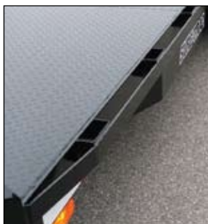
Stake Pockets & Rub Rail – Full length on both sides.
