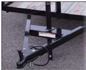
Set-Back Tongue Jack - Clearance for tailgate and SUV rear doors. (Optional)
